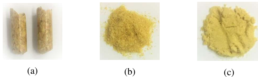
Figure 4.2 – Images of PP biomass: (a) original; (b) 106-300 \mu\text{m} ; and (c) 106 \mu\text{m} .
