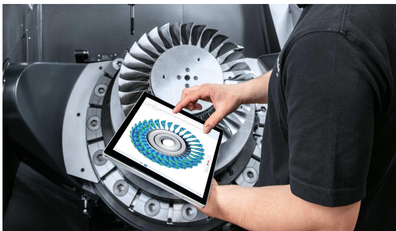
Figure 8 – Digital twin of a blisk in the gemineers software.
