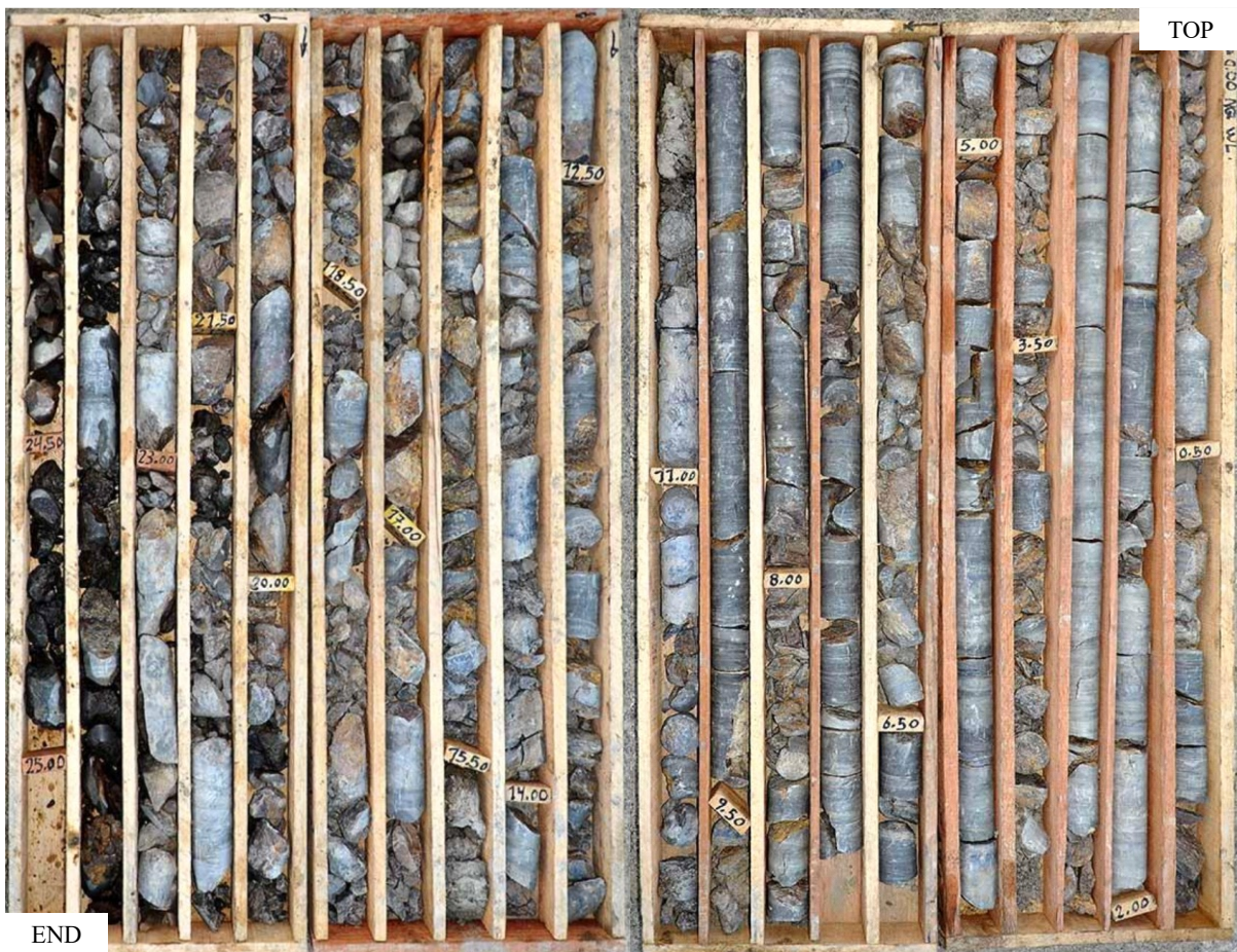
Fig. 4. Drill core S-401 showing the rock mass quality.
