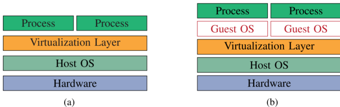
Figure 7 – Simplified architecture. (a) Container. (b) Virtual Machine
