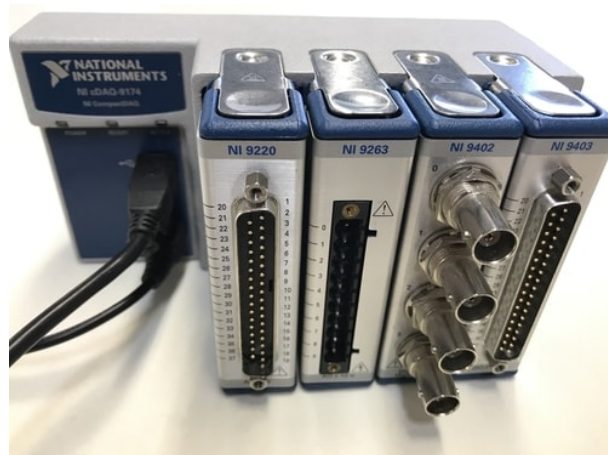
Figure 25 – Data acquisition device NI-9220 and chassis NI cDAQ-9174.
