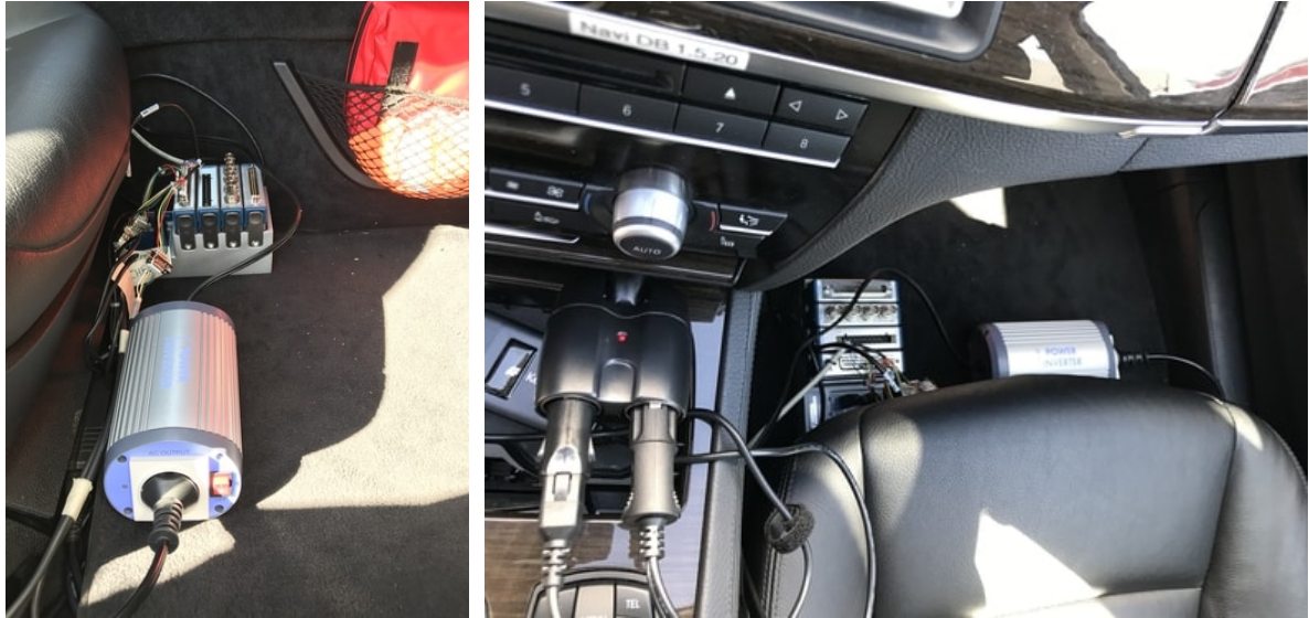
Figure 55 – Data acquisition device fixed on the feet area of the front passenger's seat.
