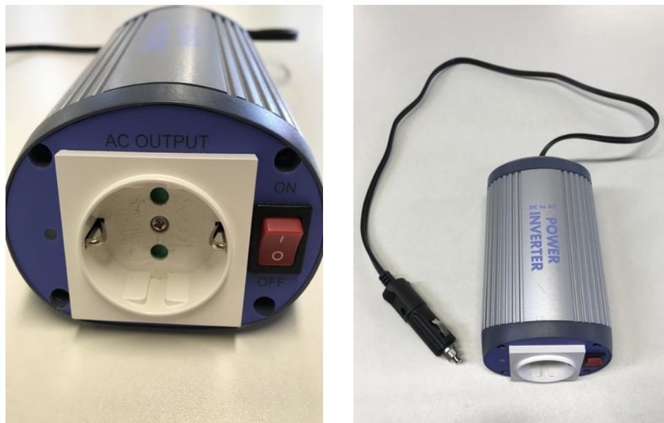
Figure 54 – DC-AC inverter used to power the data acquisition device.
