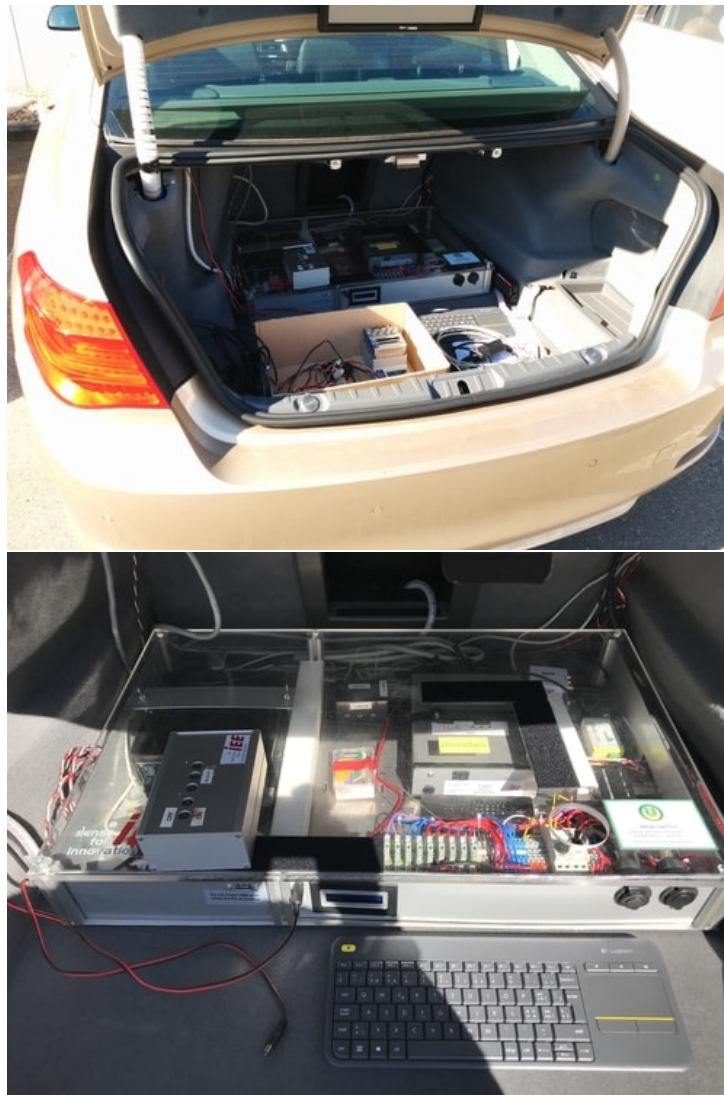
Figure 52 – Power control system built-in into the vehicle's trunk.
