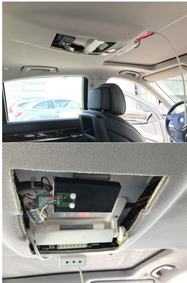
Figure 53 – Positioning of the radar behind the vehicle's headliner (top) and closer view of the radar in its mounting base (bottom).
