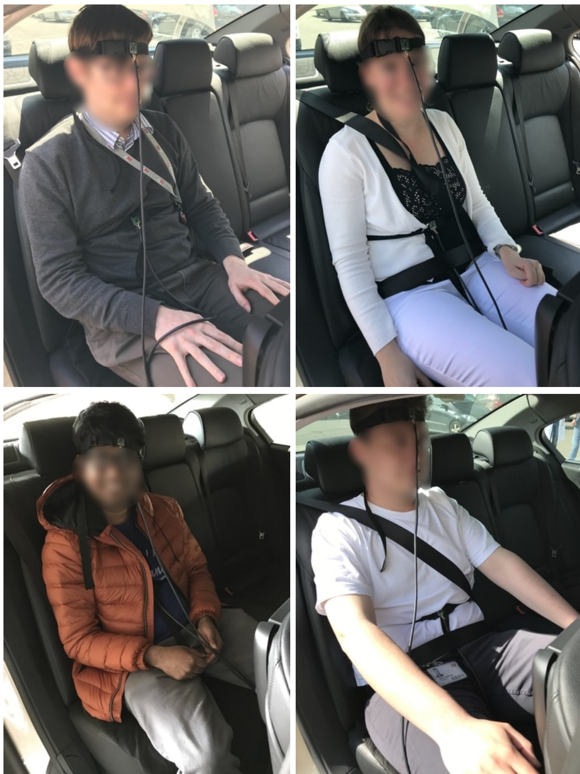
Figure 65 – Test subjects wearing accelerometer belts (head and chest).
