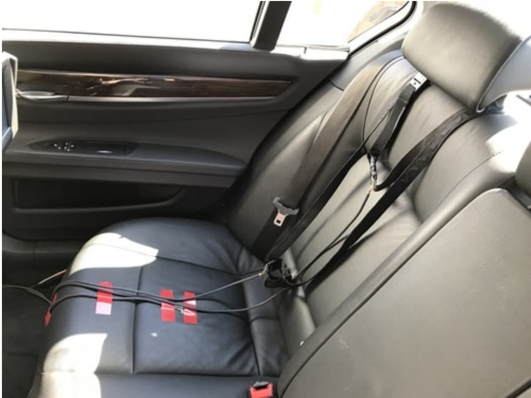
Figure 56 – Positioning of the accelerometer belts on the back right seat of the vehicle: one belt attached to the seat and two belts to be placed on the passenger.
