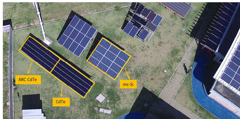
FIGURE 1 Aerial image of the three PV systems analyzed in this study (mc-Si, CdTe, and CdTe with ARC), which are part of the outdoor PV testing rig at the Fotovoltaica-UFSC Solar Energy Research Laboratory in Florianópolis (27°S, 48°W), Brazil [Colour figure can be viewed at wileyonlinelibrary.com ]
