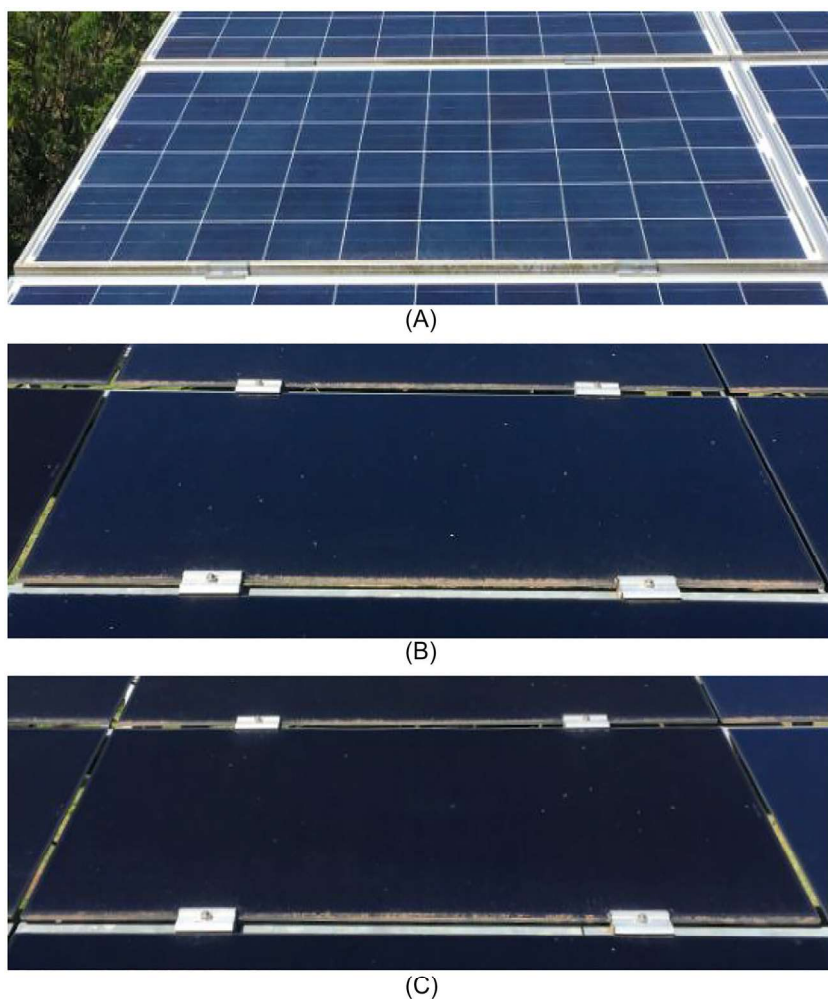
FIGURE 3 Accumulation of soiling on the modules of the three PV systems under study: mc-Si (A), CdTe (B), and CdTe with ARC (C) [Colour figure can be viewed at wileyonlinelibrary.com ]
