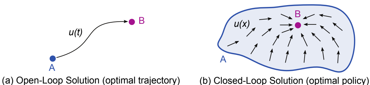
Figure 9 – Illustration of an open-loop solution and a closed-loop solution.
