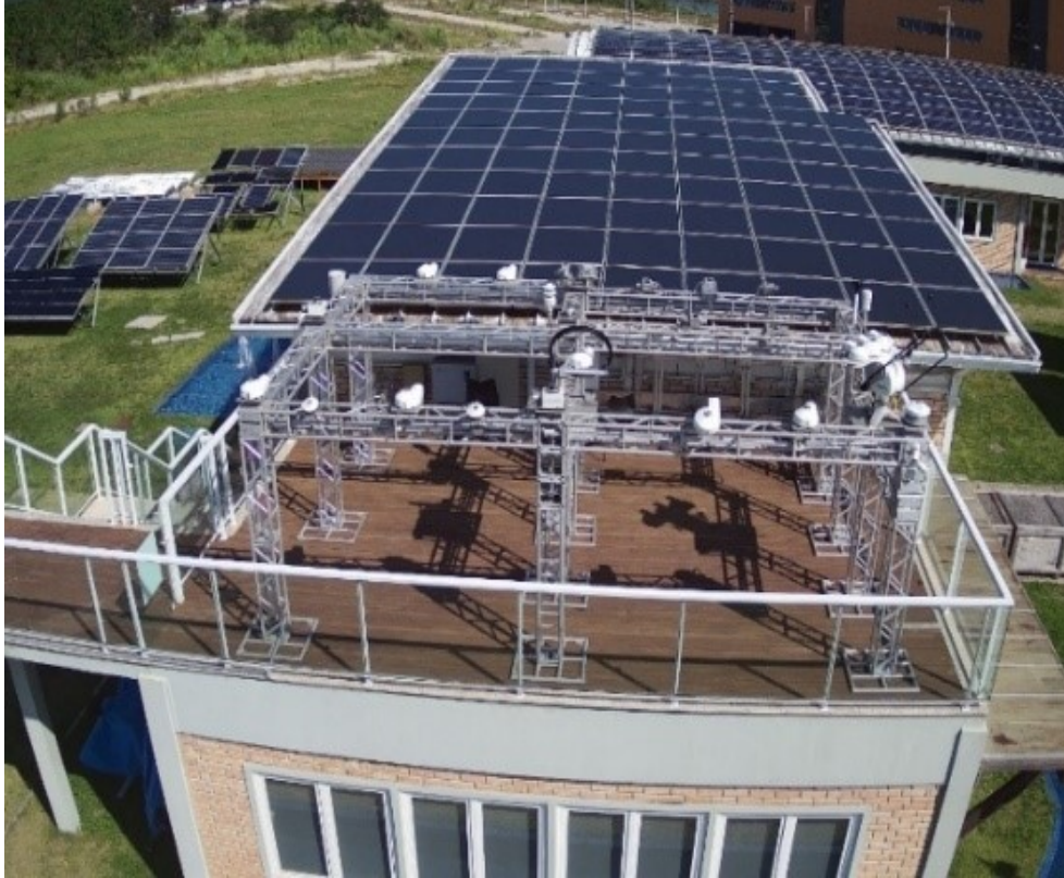
Figure 7 – The UFSC Solar Energy Research Laboratory's solar radiation measurement station in Florianópolis-Brazil.
