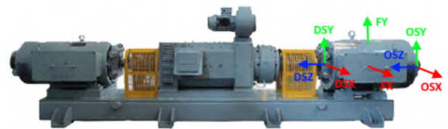
Fig. 1: Test bench for fault imposition with positions of accelerometers illustrated.
