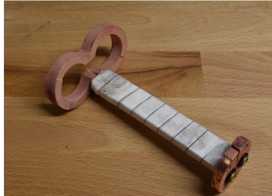
Figure 24 – Finished 2.NY 287 inductor
