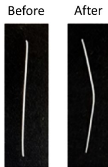
Fig. 54. Photograph of a CS-ATZ filament that had been printed with a 410 \mu\text{m} nozzle before and after undergoing cycles of deformation. It is possible to observe the expressive inelastic deformation presented by the CS-ATZ filaments after 3PB and before fracture.
