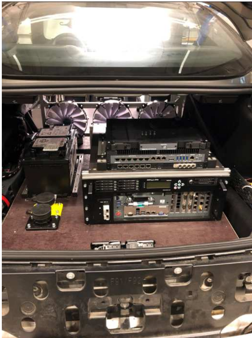
Figure 24 – Acquisition System and supply battery.
