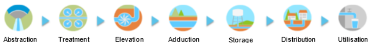
Figure 2 - Simplified diagram of a water supply system
