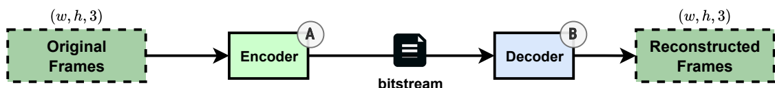
Figure 1 – Single-layer image compression model. Both the input and output images have three channels, width w and height h .
