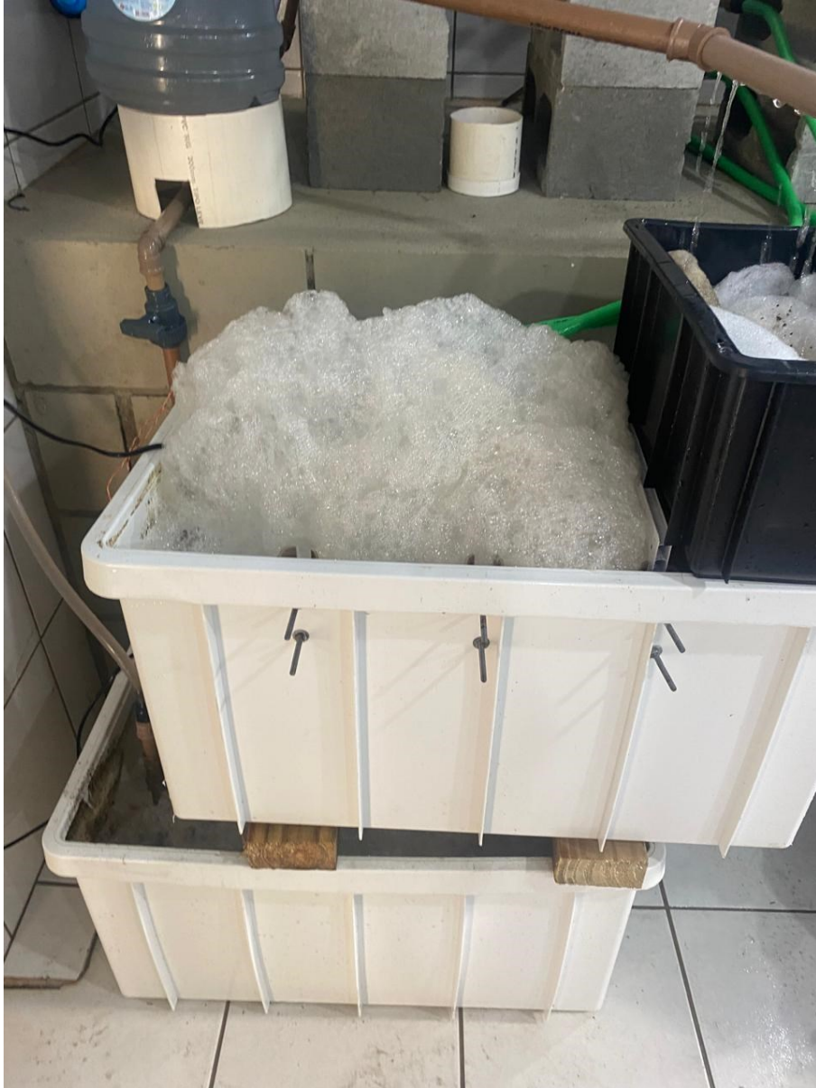
Apêndice E - Skimmer and biological reactor used for foam fractionation and nitrification. Photo by Marcelo Santana
