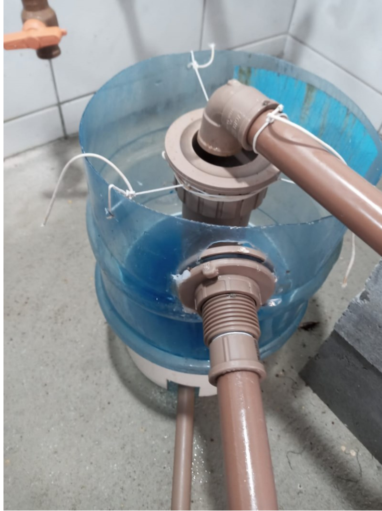
Apêndice C - Decanter used to separate solids from the recirculating water in the RAS system. Photo by Marcelo Santana
