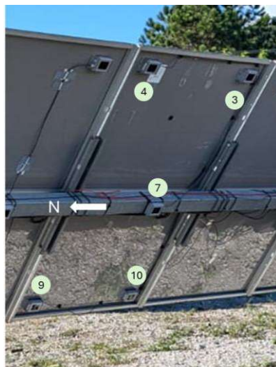
Fig. 3. Distributed reference cells for non-uniform rear irradiance measurement.
