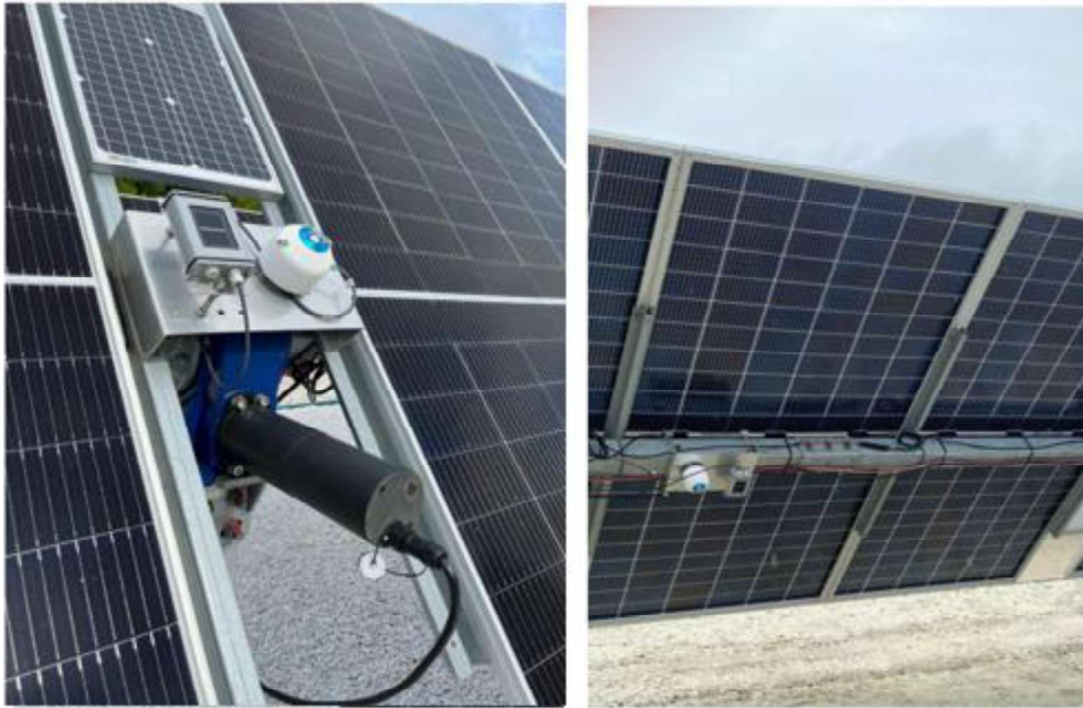
Fig. 2. Front and rear irradiance sensors (pyranometers and Si reference cells).
