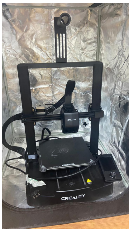
(a) Impressora de FDM Creality modelo Ender 3.
