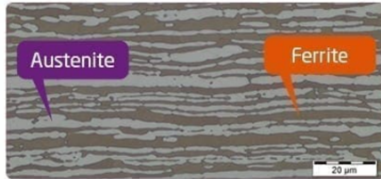
Figure 4 : Duplex Stainless Steel before welding (metal base)
