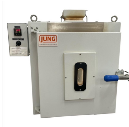
Figure 7 - Industrial furnace used for the ion exchange treatment (Jung, Brazil).
