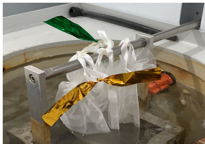
Figure 8 - Thermocycler used for the aging protocol with samples immersed and separated by groups.
