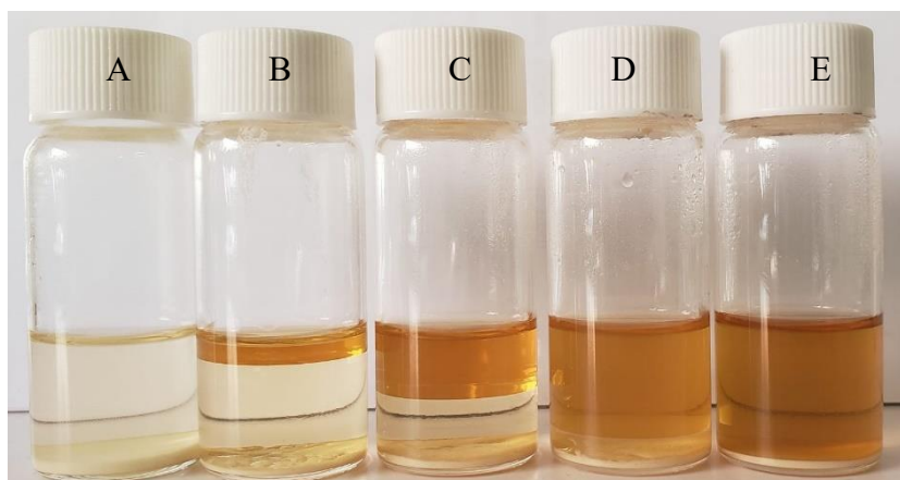
Figure 3.14. The liquid-liquid phase separation layers for different mass percentages of 2-butoxyethanol: A) 10 wt. % (homogeneous system), B) 20 wt. % (water-rich layer), C) 30 wt.% (water-rich layer and hydrotrope rich-layer), D) 40 wt.% (hydrotrope-rich layer), E) 50 wt.% (homogeneous system).
