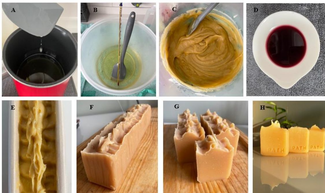
Figure 6.5. Juçara's natural soap production. (A)- oils and butter heating; (B) – melted butter and oils mixture; (C)- soap mass before additives; (D)- juçara extract (42.6% of 1,2-propanediol in 1:50 g/mL of juçara dried pulp); (E)- parchment paper-lined molds filled with soap mass; (F)- loaf of soap after 24h; (G)- soap bars; and (H)-soap bars after cure.
