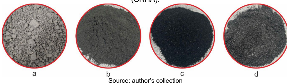
Figure 2.1 – Macroscopic appearance of the (a) aluminum salt slag (ASS), (b) hydrolyzed slag (HS), (c) rice husk ash (RHA) and (d) calcined rice husk ash (CRHA).
