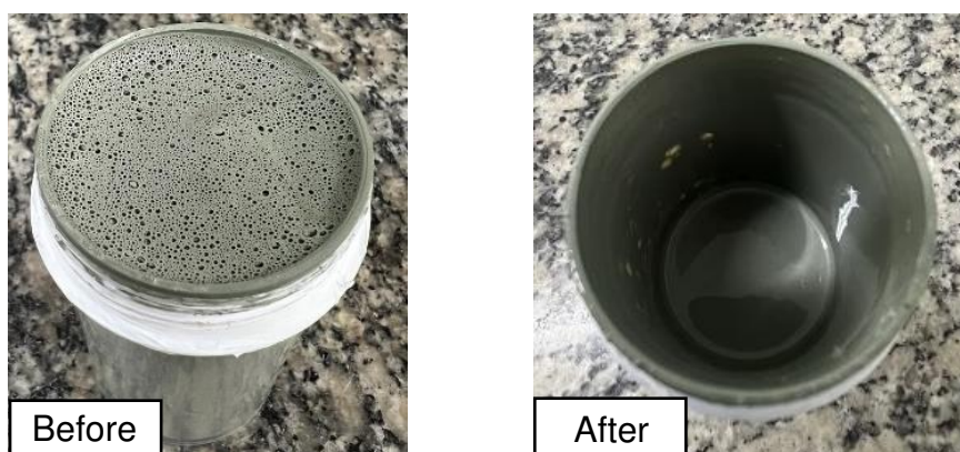
Figure 63 – Foam elimination by using defoamer, before and after addition.
