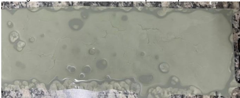
Figure 64 – Functional anode attempt of composition FA1.
