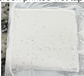
Figure 51 – Screen printed wet tape with bubbles.
