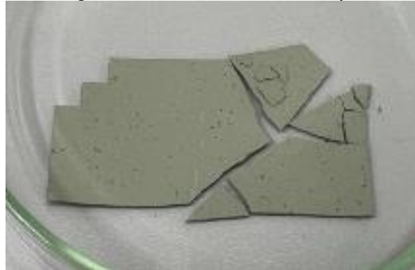
Figure 73 – SA3 debinded tape.
