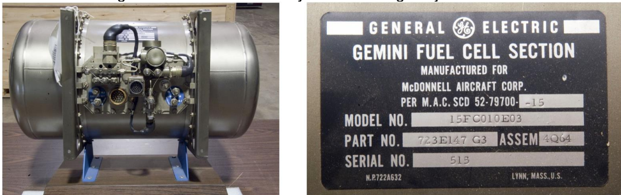
Figure 1 – Fuel cell used by NASA during Project Gemini.
