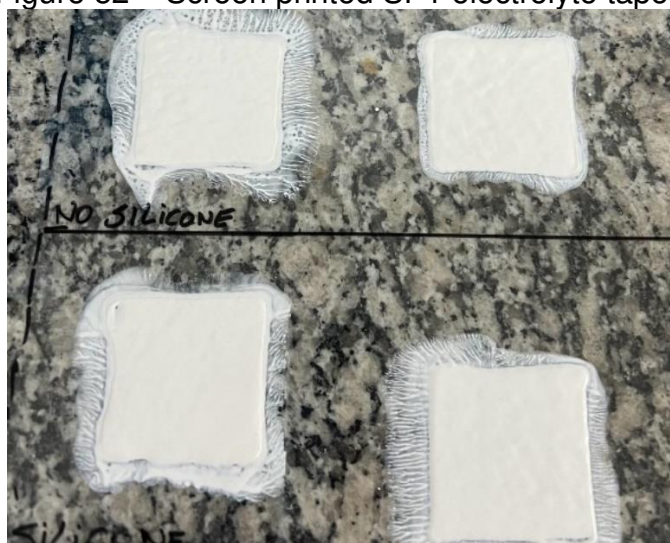
Figure 52 – Screen printed SP1 electrolyte tapes.
