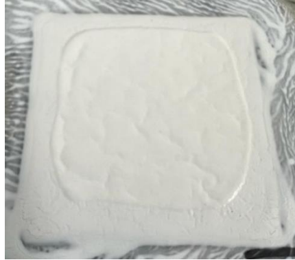
Figure 53 – Screen printed tape drying.
