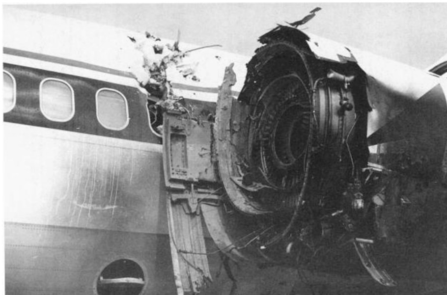
Figure 7 – Uncontained failure due to a manufacturing induced anomaly
