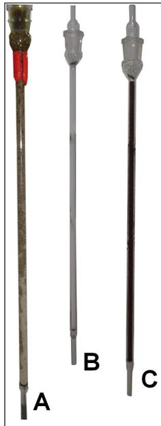
**Figura 3.3** – Coluna recheada com: A – resina C150; B – resina A860S; C – resina PCR 642Ca.
