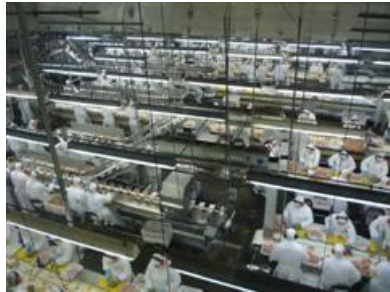
Figure 5 – Poultry cuts: the main product of the slaughterhouse (although it is also equipped for whole chicken). After cooling, is the removal of viscera (who follow parallel processing line) head, trachea and lungs. In parallel lines, several types of cuts are made (manual and automatic lines).
