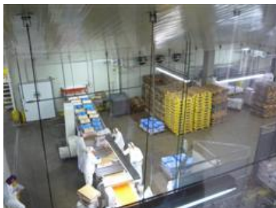
Figure 8: Packaging Sector. After passing through the freezing chamber, the other cuts are accommodated in special packaging, pass through metal detectors, inventory control (bar code) and end labeling.
