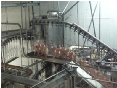
Figure 3 – End of first stage: after hanging, stunning, bleeding and plucking, the birds pass through the federal inspection and move on to next step
