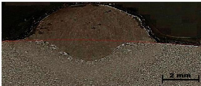
GMAW Imp. Tensão,  $V_s=30\text{cm/min.}$ ,  $I_m=143\text{ A}$ ,  $E_s=3,32\text{ kJ/cm.}$ ,  $P=1,35\text{ mm}$
