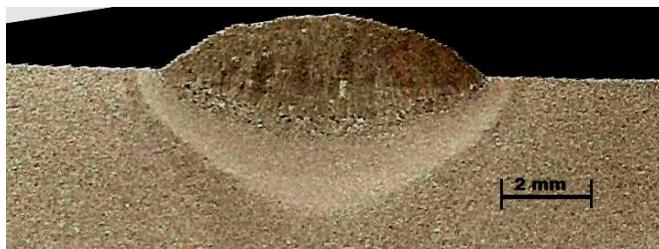
FCAW-S Imp. Tensão,  $V_s=30\text{cm/min.}$ ,  $I_m=139\text{ A}$ ,  $E_s=4,9\text{ kJ/cm.}$ ,  $P=1,47\text{ mm}$
