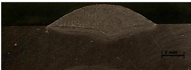
GMAW Pulsado,  $V_s=30\text{cm/min.}$ ,  $I_m=140\text{ A}$ ,  $E_s=8,4\text{ kJ/cm.}$ ,  $P=1,1\text{ mm}$
