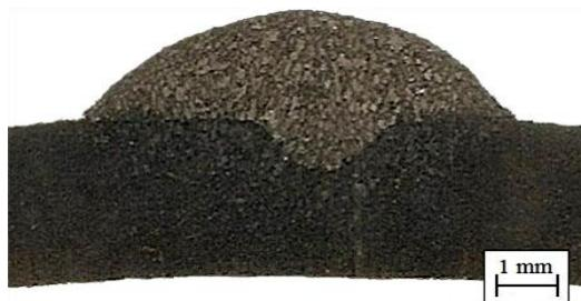
Foto A ( $I_m = 75A$ ;  $V_s = 25 \text{ cm/min.}$ ;  $E_s = 4,2 \text{ kJ/cm}$ ;  $P = 1,0 \text{ mm}$ )
