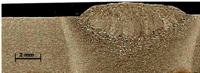
FCAW-S Pulsado,  $V_s=30\text{cm/min.}$ ,  $I_m=140\text{ A}$ ,  $E_s=8,3\text{ kJ/cm.}$ ,  $P=1,85\text{ mm}$
